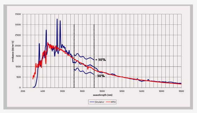
\* Above is a graphical demonstration of adjusting zone 2 of the 'N-Zone' simulator. Unlike the Unisim simulator, there is no overlap between spectral zones.
